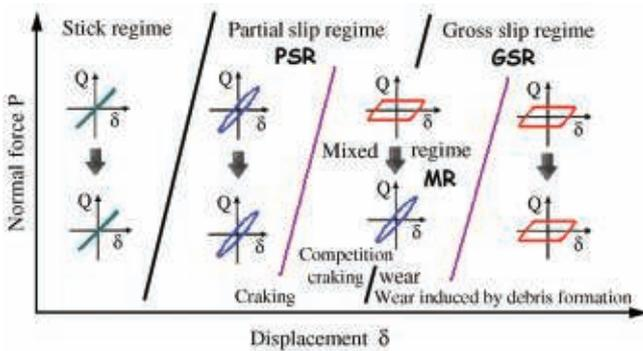
Fig. 1. Running condition and material response fretting maps [11].
