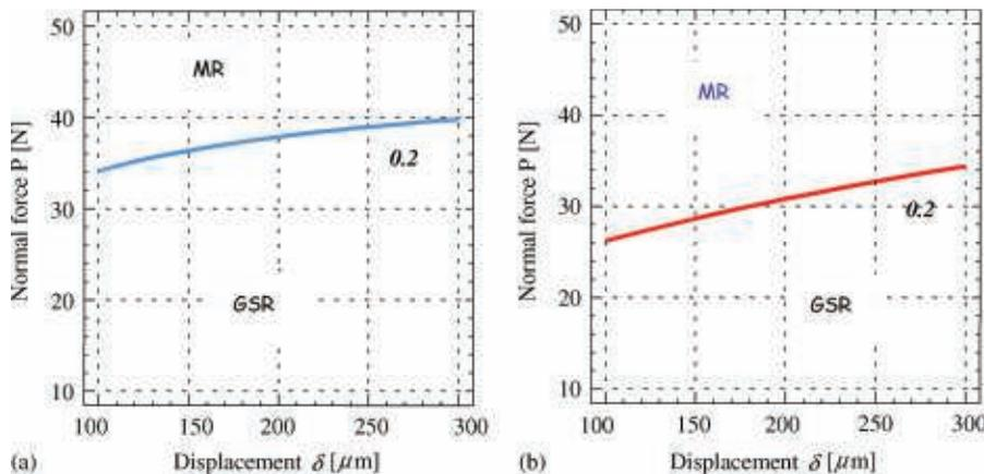
Fig. 7. Running condition fretting maps ( $f=15$  Hz,  $N=5000$  cycles): (a) smooth surface; (b) textured surface.
