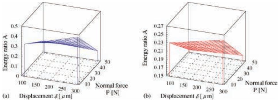
Fig. 6. Response surfaces for the energy criterion  $A$  ( $f=15$  Hz,  $N=5000$  cycles): (a) smooth surface; (b) textured surface.
