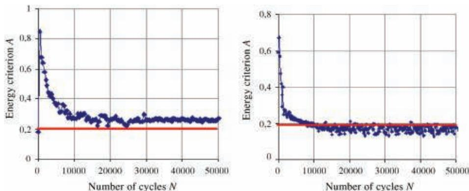
Fig. 8. Energy criterion  $A$  ( $P = 10\text{ N}$ ,  $\delta = 100\ \mu\text{m}$ ,  $f = 10\text{ Hz}$ ) (run no. 1): (a) smooth surface; (b) textured surface.
