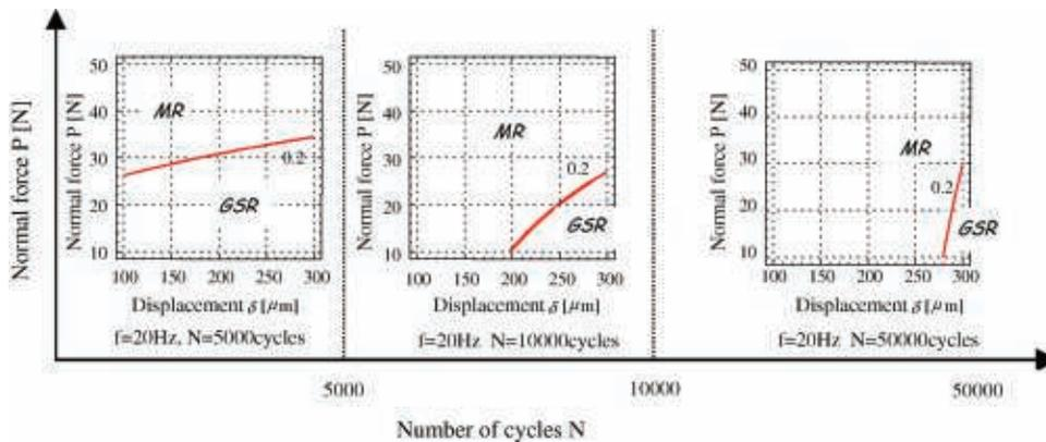
Fig. 10. The running conditions fretting maps for the textured surface.
