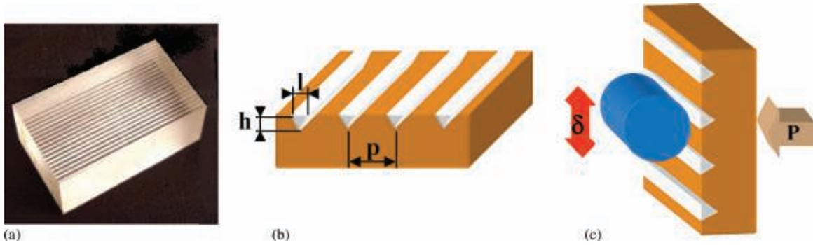
Fig. 2. Textured surface: (a) photograph; (b) schema; (c) schema of the contact.
