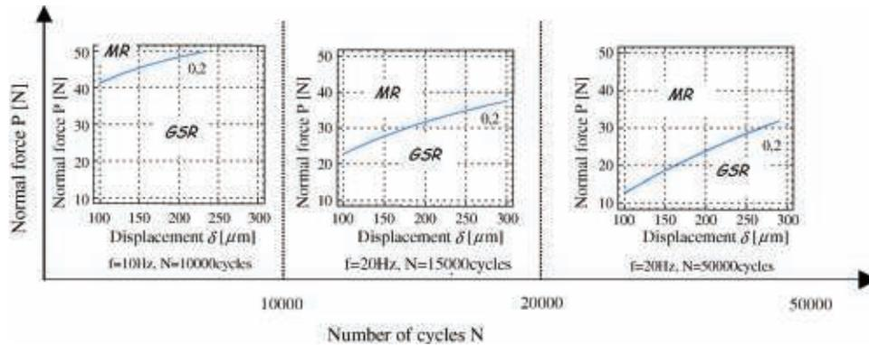
Fig. 9. The running conditions fretting maps for the smooth surface.
