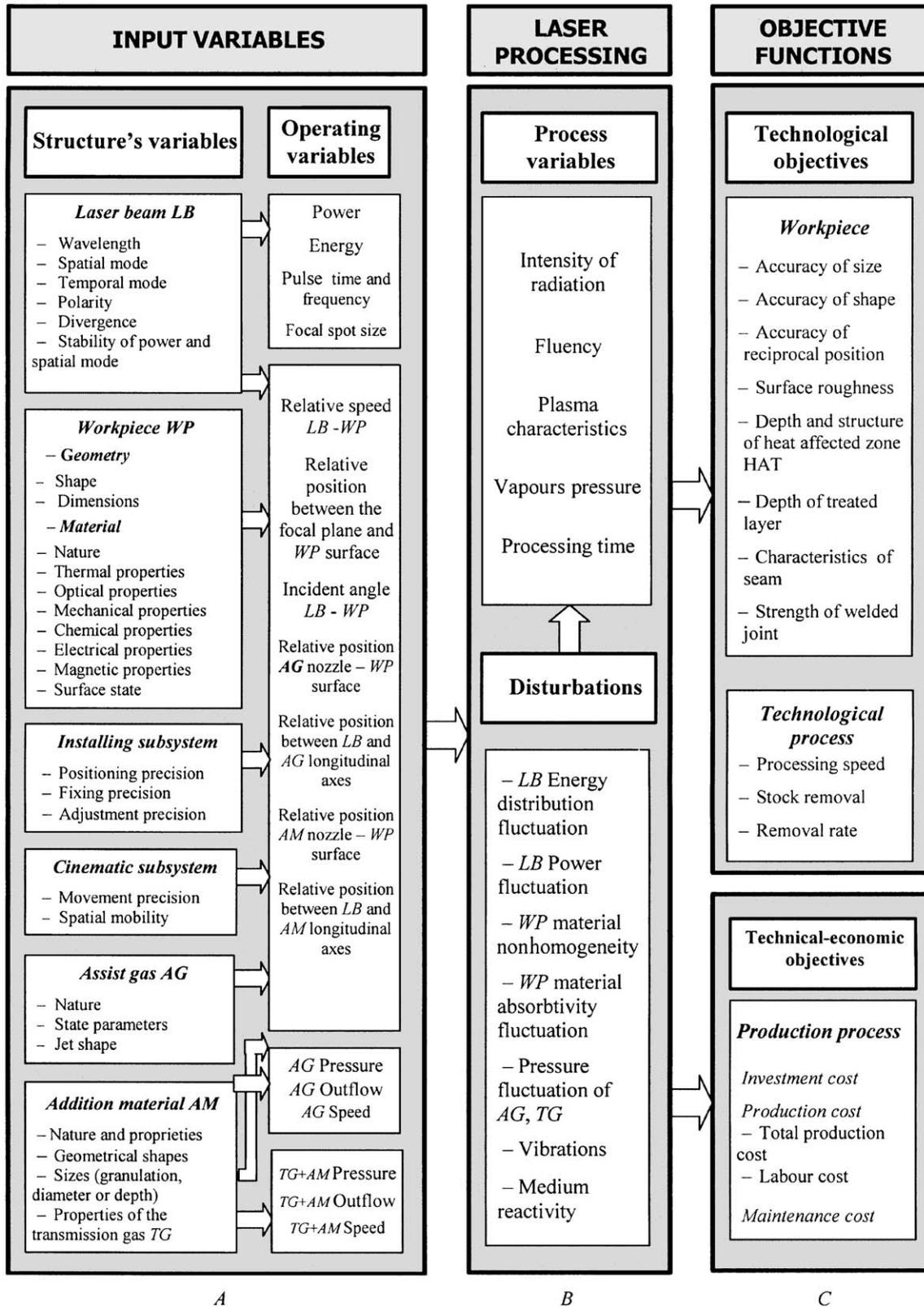
Fig. 1. Characteristic variables of material laser processing.
